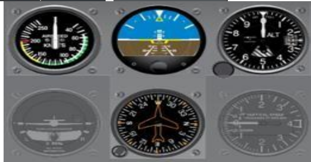
(a) Basic 'T' flight instrument configuration
