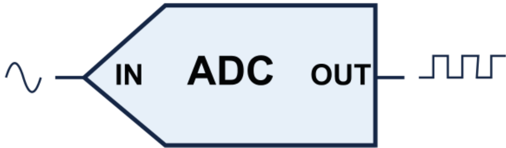
Figure 3-3. Symbol for an analog to digital converter.
