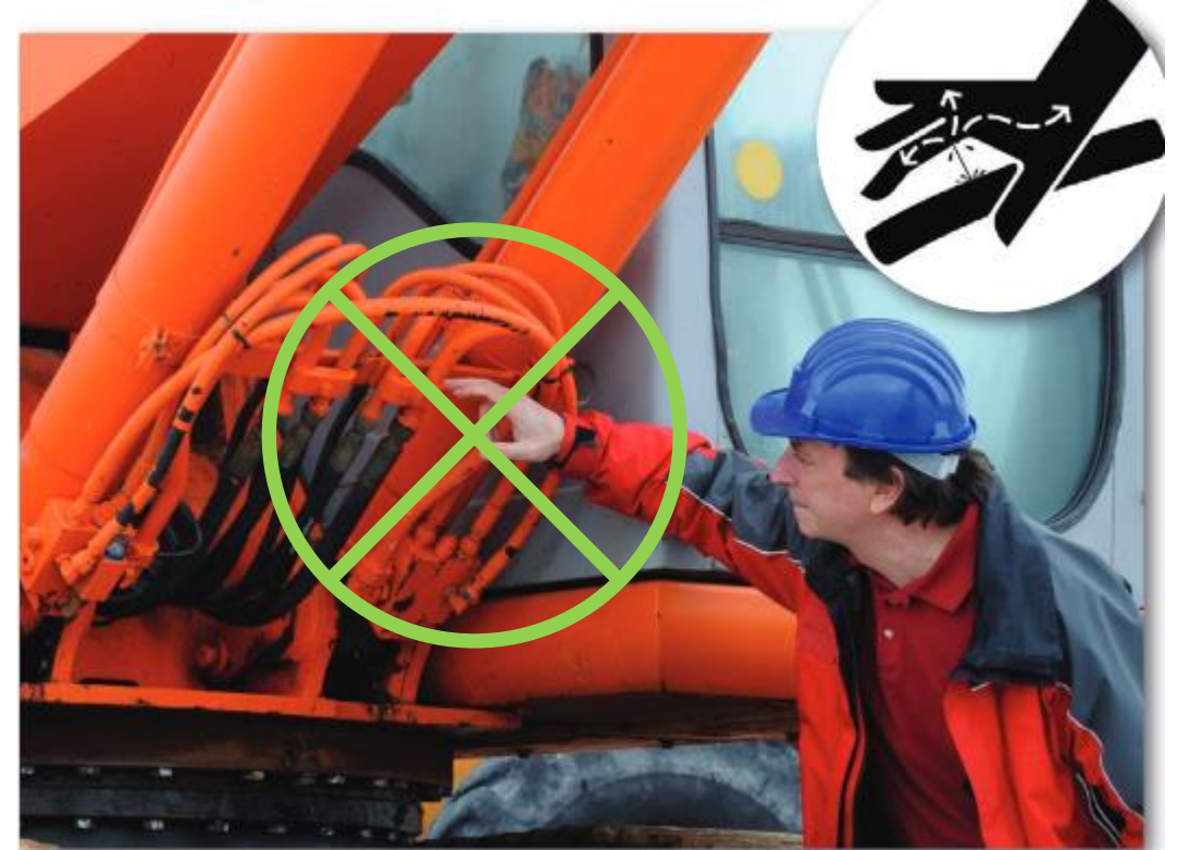
This is NOT the way to check for leaks!
