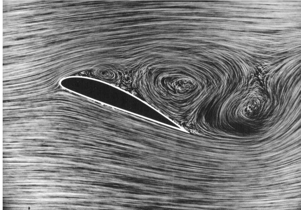
Airflow separating from a wing at a high angle of attack - 1915ca_abger_fluegel_(cropped_and_mirrored)
