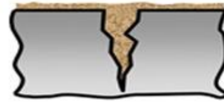
1 Crack filled with dirt
