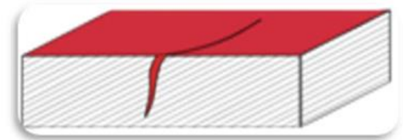
Application of the penetrant (Red)
