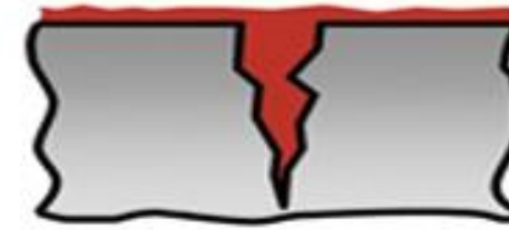
3 Application of penetrant
