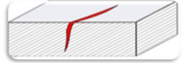
Application of the penetrant (Red)
