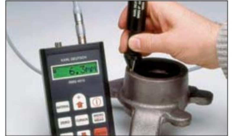
Measurement of a normal crack on a small area
